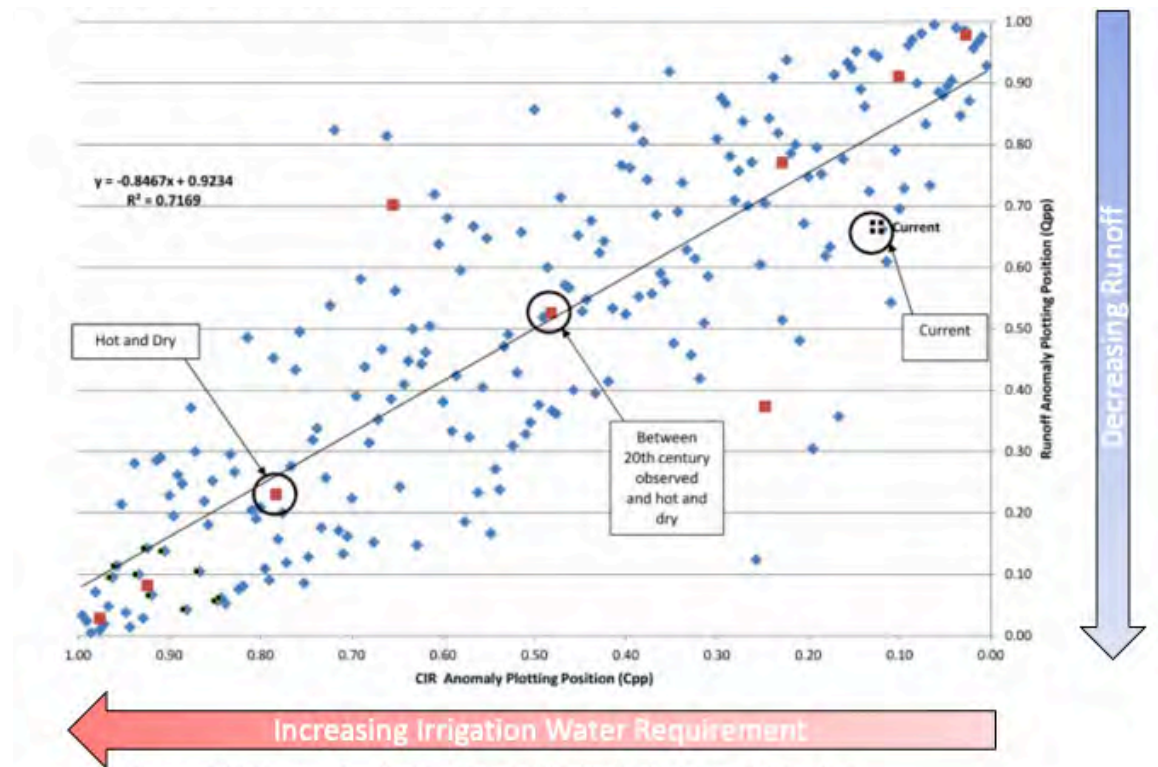
Figure 6. Three climate scenarios selected for use in the Technical Update models bracket the range of Runoff Anomalies and Crop Irrigation Requirements predicted by a large number of climate models/runs.
